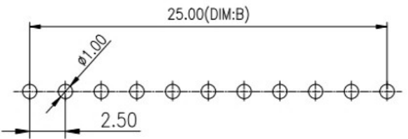
Recommended P.C.B Layout Layout Tolerance=+/-0.05mm
